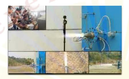
India's 1st private-built cryogenic rocket engine was test-fired by skyroot aerospace in Hyderabad. The Hyderabad-based space technology test-fired the Dhawa-1 India's first privately designed and developed cryogenic rocket engine, the engine is set to power the upper stages of the upcoming Vikram-2 orbital launch vehicle, developed using 3D printing with superalloy, the Dhawan-1 is a 'Made-in-India cryogenic engine.
